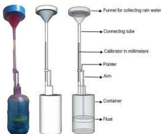
Fig.(2) Rain gauge device for measuring rainwater falling in the field [14].
