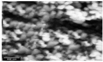
Fig. (2) SEM images of Nano K- Silicate
