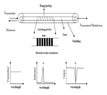
Fig. 1: Spectra of the transmitted, reflected, and output waves as well as the fiber Bragg grating structure.
