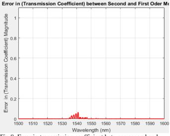
Fig 8: Error in transmission coefficient between second and first order model.
