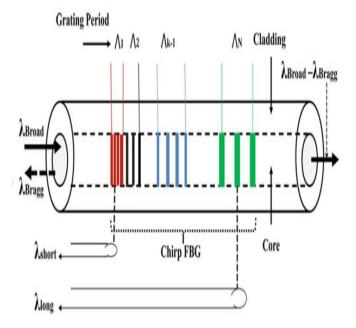
Fig. 2: A chirped FBG's configuration as a dispersion compensator.
