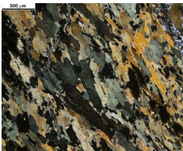
Fig (11) Photomicrograph in the present foliated amphibolite showing well developed foliation represented by amphibole minerals. (X.P.L).
