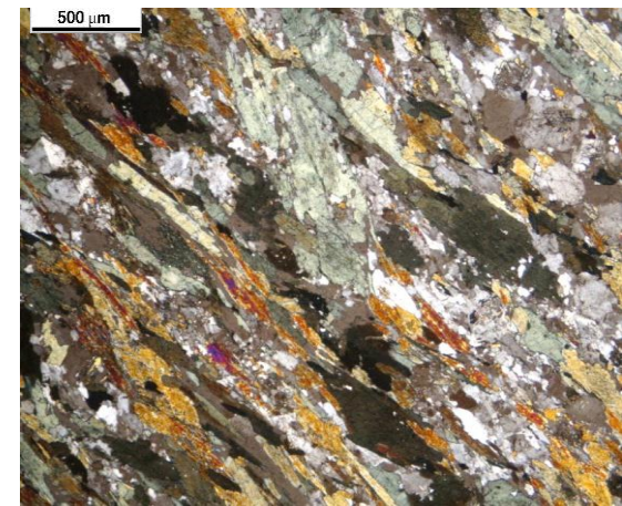
Fig (10) Photomicrograph showing well developed foliation in the coarse grained flaser metagabbros. (X.P.L).
