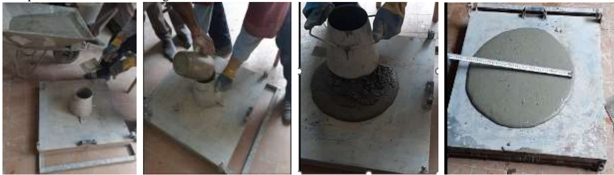
Fig. (4) Flow Test (T500) Procedures.
